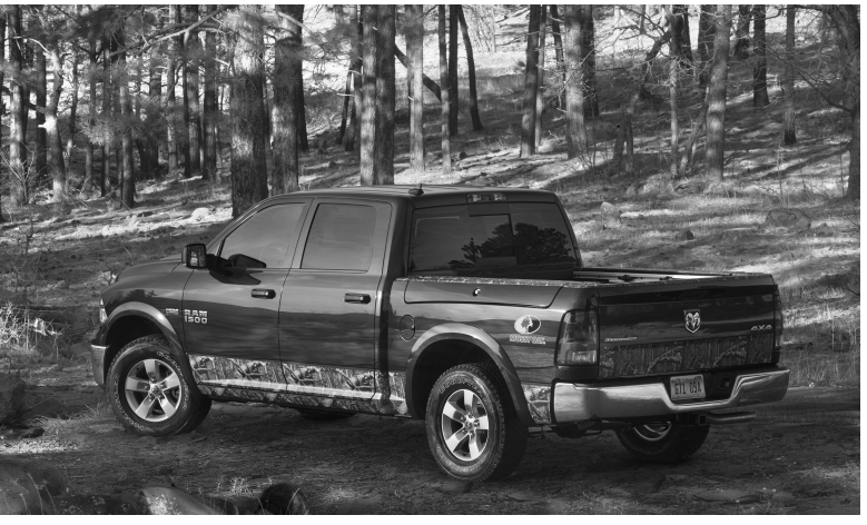
Ram 1500 was praised for its new EcoDiesel V-6 engine, new eight-speed automatic transmission and standard rear coil suspension. PHOTO COPYRIGHT CHRYSLER GROUP LLC.
